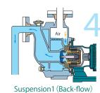
Liquid flows back after stop the operation, but our original siphone cut structure holds the liquid quickly and remains enough self-priming liquid in the casing.
