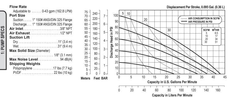
NOTE: Performance based on the following: elastomeric fitted pump, flooded suction, water at ambient conditions. The use of other materials and varying hydraulic conditions may result in deviations in excess of 5%.
