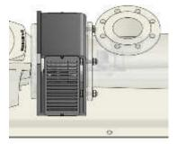
Hermetic Lantern. This particular capsulated lantern is equipped with gaskets on the covers to isolate the outer part of the seal, the compartment and the plug-in shaft.
