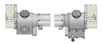
Tangential coupling flanged or with threaded coupling for fluid drainage in the body or hopper. The tangential structure avoids product residue and stagnation.
