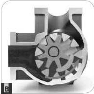
The pump is equipped with one shaft seal or with magnetic coupling only, and has the possibility of a heating jacket around the casing in one cast. The full performance is available in either direction of rotation and the casing can be rotated and delivered with 90° or 180° (in-line) ports. A safety relief valve against over-pressure is incorporated in the pump. This is a heavy duty construction optimized for rare maintenance.
